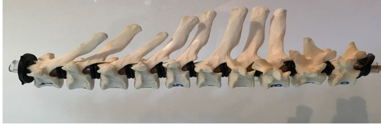
Fig. 1 Canine vertebrae, with the vinyl tubing inserted through the cavities and the rubber O-rings between each vertebrae, prior to complete immersion into the gel.
